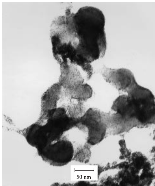
Fig. 2 TEM of Pt oxide nanoparticles dispersed on PPy/PSS particles
