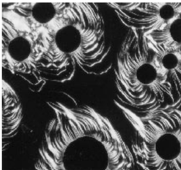
Fig. 1 Polarized optical micrograph of the TGBA phase on heating to 143.8 °C; magnification \times 100
