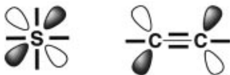
Fig. 7 Comparison (diagrammatic, not stereochemical) of the electronic components of sulfide \text{S}^{2-} and acetylide \text{C}_2^{2-} available for bonding participation in metal clusters. Both have four donor electron pairs marked as heavy lines (for \text{C}_2^{2-} these are the terminal \sigma pairs and the two \pi bonding pairs) and both have empty orbitals marked as lobes, being d orbitals at S and \pi^* orbitals on \text{C}_2^{2-} : not all of these empty orbitals are shown.
